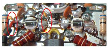
After this you have to **align the 500 ohm pot** to a **total current consumption of the PA** of about **2A** (only PTT, without any RF input signal). This BIAS works great.
