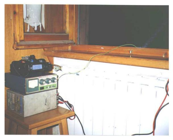
The yellow / green wire, about 1-meter long and actually forming part of the antenna, joins the antenna tuner out to the mast base (you can barely see the mast in the dark). A heavy brown wire connects the antenna tuner ground to the heating system radiator, acting as earth (you can see that wire adjacent to the radiator knob). It is very important to have a good counterpoise for the antenna, so the wire must be thick and as short as possible.
