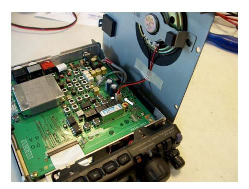
It works best if you also remove the bottom cower by removing these 9 screws. Be careful with the battery compartment lock!
