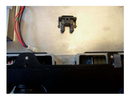
Disconnect the four cables from the front and RF/amplifier unit. The cable from the front can not be just pulled out of the connector, you have to lift the brown "lock" be careful, do not break the hinges.
