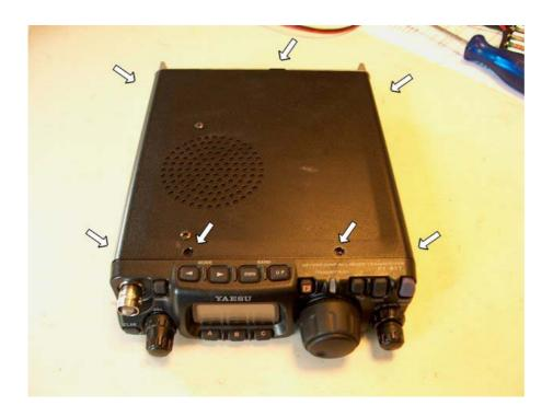
Remove the cover carefully and disconnect the speaker wires.
