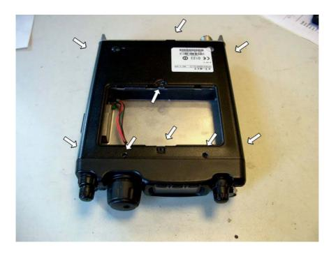
Remove the bottom cover and this little plastic part and the springs, so you will not loose this or the springs.
