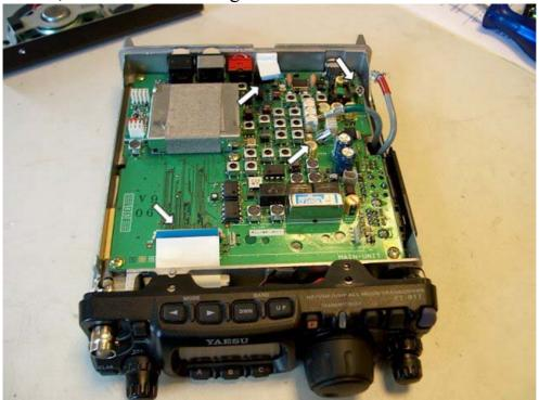
Now you van remove the 5 screws that hold the PCB and then you can lift the PCB out of the housing.
