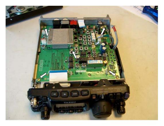
Turn the PCB upside-down and locate the 4.7 Ohm Resistor. Solder a resistor parallel to this one to increase the current.
