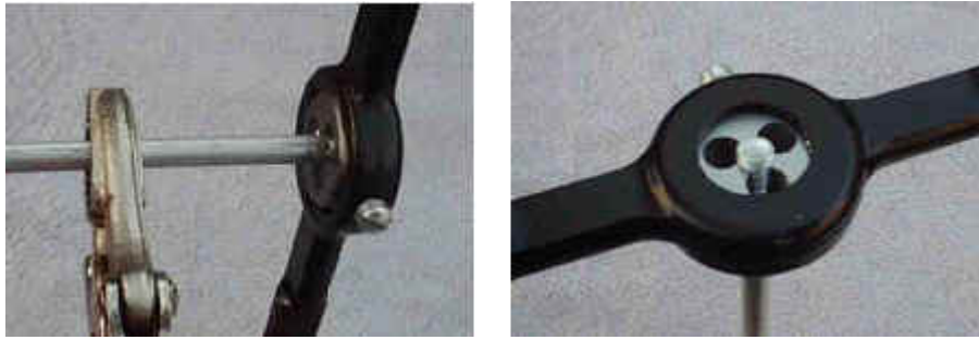
Figure 13: Cutting the threads
