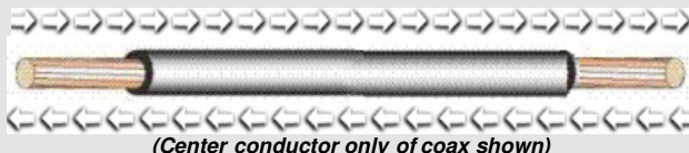
Rf moves both ways in center conductor of coax!
