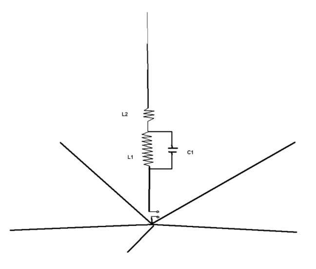
On 40m, the RF "sees" the lower coil as the high impedance path, and so goes via the capacitor to the upper coil, and on to the rest of the vertical. Because of the "shortening" effect of the series capacitor, the upper coil is required to bring the antenna back to 1/4 w/l resonance.
