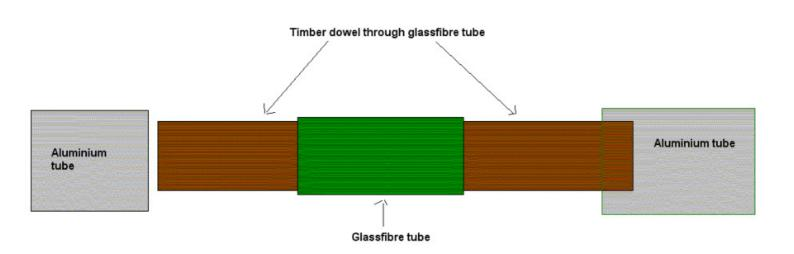
The next step was to push one end of the dowel into the 6ft length of aluminium tube, and the other end into another length of aluminium tube about 18 ft long. I then got a glassfibre tapered tube (one of my store of Quad arms) and ran aluminium wire up through it, and out the top a further foot or so.
