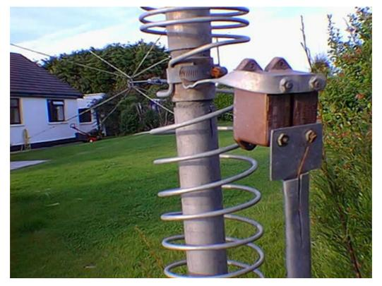
I next connected my trusty MFJ SWR analyser, and the battle commenced. By tapping the coils with the fly leads, and moving the hoseclips up and down, to stretch, or compress the coils, I eventually got resonance on 80m and 40m. The SWR was about 1.5:1 on 80m, and a bit better on 40m.
