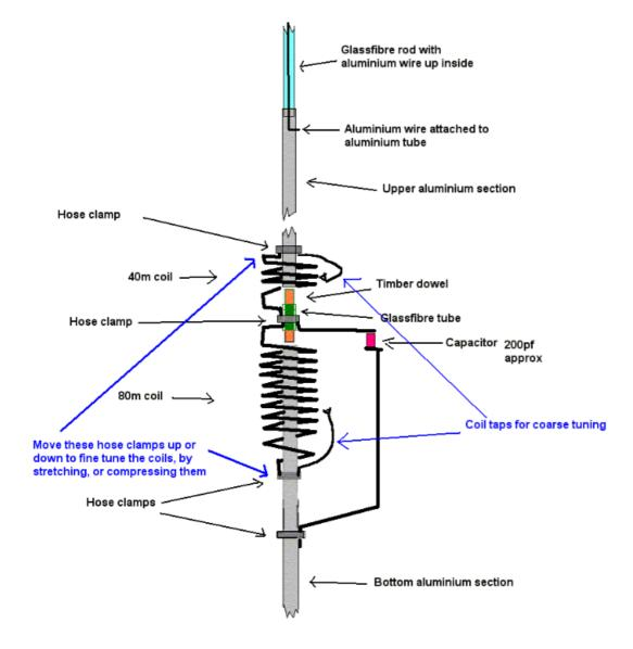
I got a pair of capacitors which were marked as being 100pf each. I mounted these in parallel as shown in the pics. When I measured their value using the MFJ SWR analyser, the value at 3.6mHz was 250pf. Having got the antenna raised to the vertical position, I guyed it with three lengths of nylon twine.
