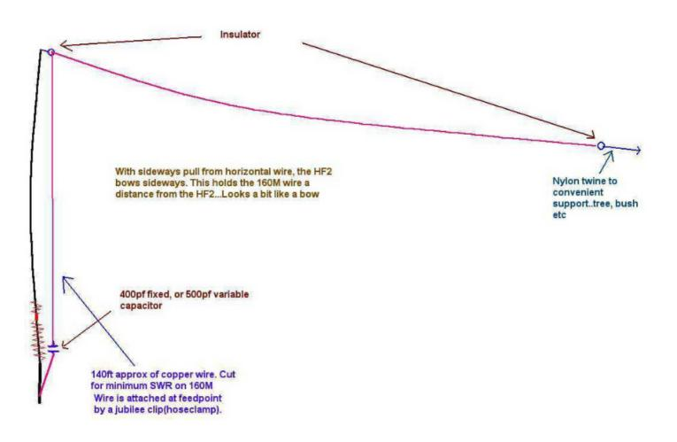
The other option would be to use a fixed wire length, and a 500pf variable capacitor. This would allow you to tune anywhere in the band.
