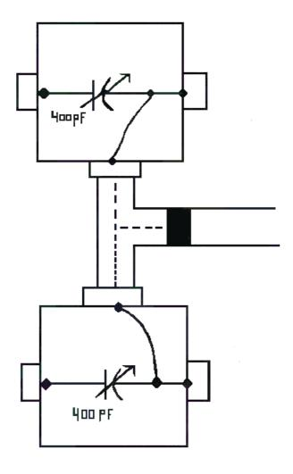
The trimmer values are aprox the vaue shown above. However I've used ARCO 468 for the 160m loop and ARCO 467 trimmers for the 80m loop, with great success. RG8X can be of random legth. I usually cut them to fit between the boxes. The lead to the receiver can be of any length.
