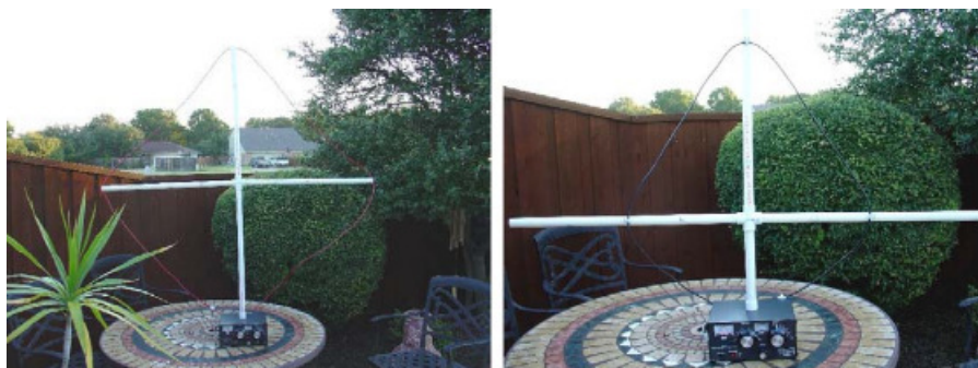
13-ft 10ga 30-20m wire loop & MFJ-936B 7-ft 10ga 20-15m wire loop & MFJ-936B
