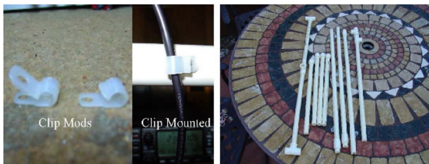
Nylon clip mounting details Unassembled MFJ-932 CPVC support
