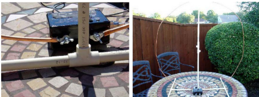
MFJ-932 copper loop attachment MFJ-932 and 10-ft 20-15m copper loop
