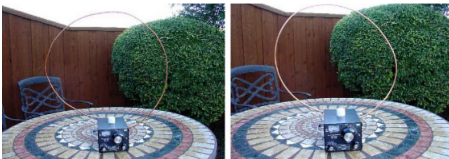
6-ft 20-15m copper loop and MFJ-935B 5-ft 17-10m copper loop and MFJ-935B
