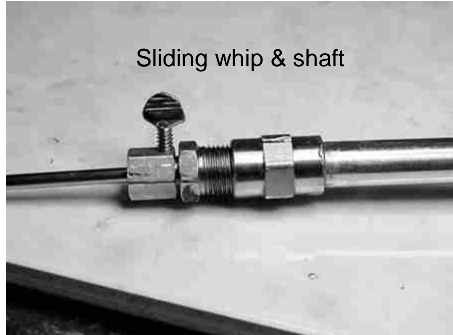
1/8 Compression-to-1/8NPT Adapter Drilled & tapped for #6 thumb screw
