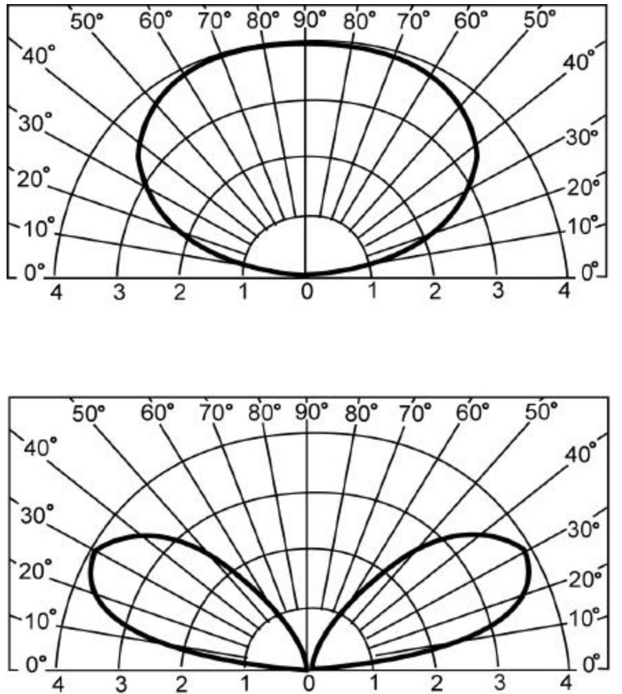
The top radiation pattern is that of a half-wave horizontal antenna one quarter wavelength above the ground and the bottom pattern is that of a half-wave horizontal antenna, one half wavelength above the ground.
