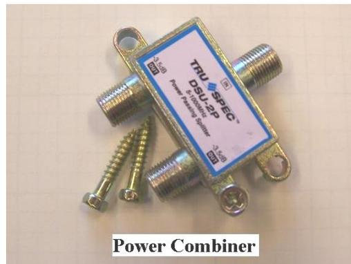
A **Power combiner** adds the signals from both dipoles together. The combined signals are then sent to the receiver.
