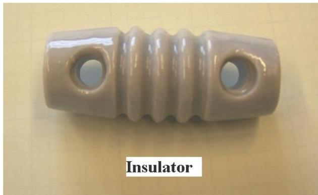
**Insulators** support the antenna wires while isolating the received signals from ground. Six insulators are used for the antenna, one at the feed point in the middle of each dipole, and one on each end.
