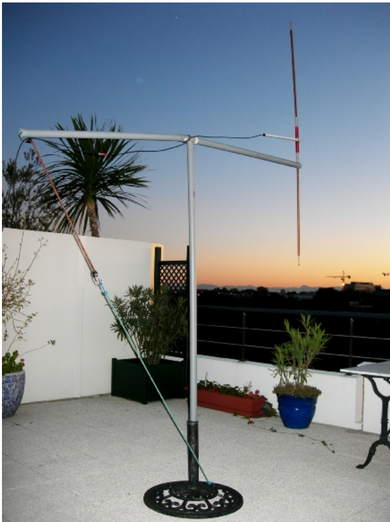
Installation of the antenna on my terrace - mounted 2 m off the ground
