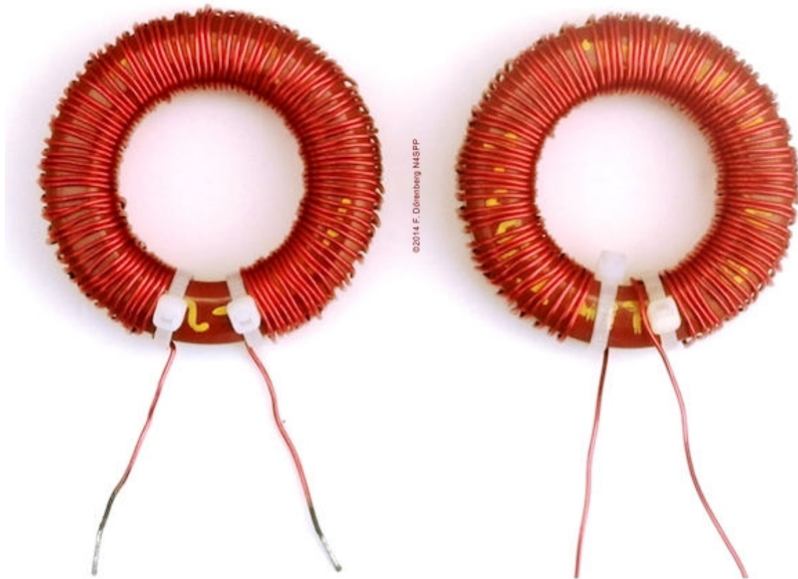
The two 117 \mu\text{H} loading coils, 95 turns wound on T200-2 iron powder cores
