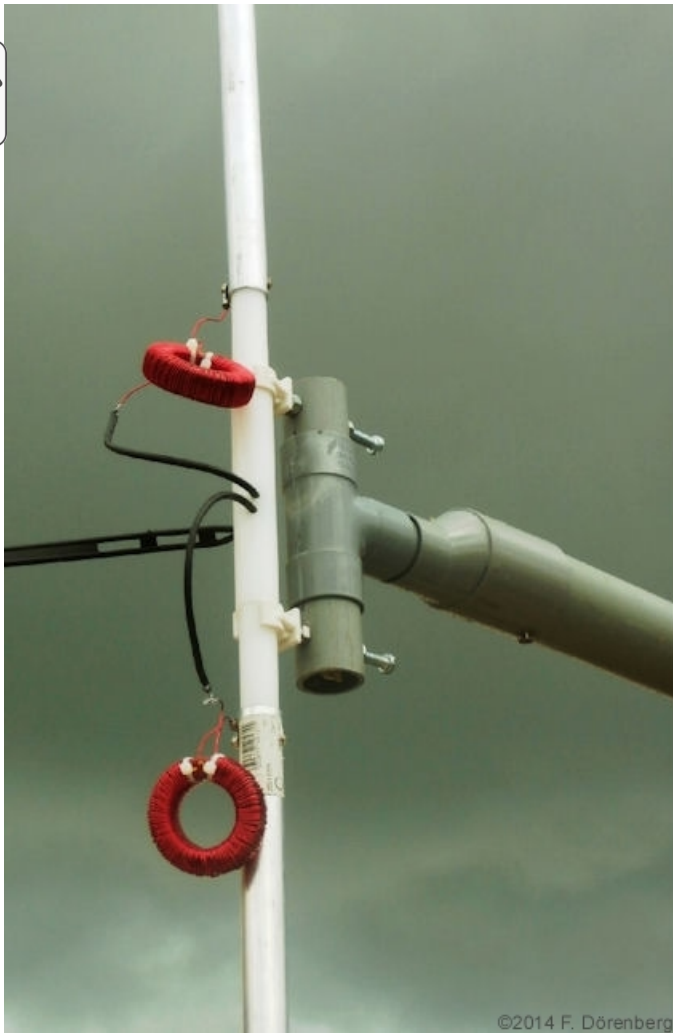
Two loading coil configurations: 117\ \mu\text{H} on iron powder core (left) and 77\ \mu\text{H} on PVC core (right)
