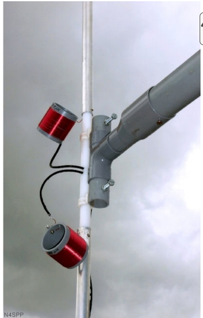
Two loading coil configurations: 117\ \mu\text{H} on iron powder core (left) and 77\ \mu\text{H} on PVC core (right)
