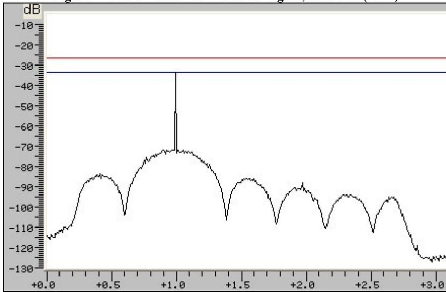
**6: Manual Notch Filter (MNF) stopband attenuation and bandwidth.** In this test, an RF signal is applied at a level slightly more than 70 dB above MDS. The test signal is offset 1 kHz from the receive frequency to produce a test tone. The MNF is carefully tuned to null out the tone completely at the receiver audio output. The stopband attenuation is equal to the difference between the test signal power and MDS.
