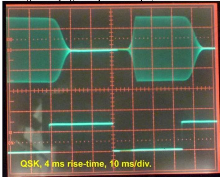
**22b. CW QSK recovery test:** This test was devised to address Yahoo! Group reports that CW QSK (full break-in) does not work well when using the internal keyer at speeds > 12 wpm. If a string of dits is transmitted at speeds > 12 wpm, the receiver does not recover between dits.
