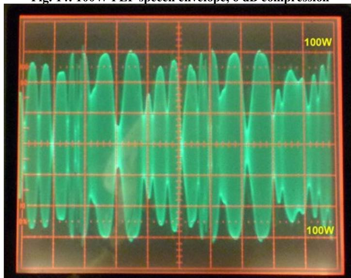
**17a: SSB ALC overshoot:** Reports of ALC overshoot in the IC-7410 Yahoo! Group led to an investigation of this issue. A test was performed in which white noise was applied via the USB port, and the RF envelope observed on an oscilloscope terminated in  $50\Omega$  and connected to the IC-9100 RF output via a 50 dB high-power attenuator.
