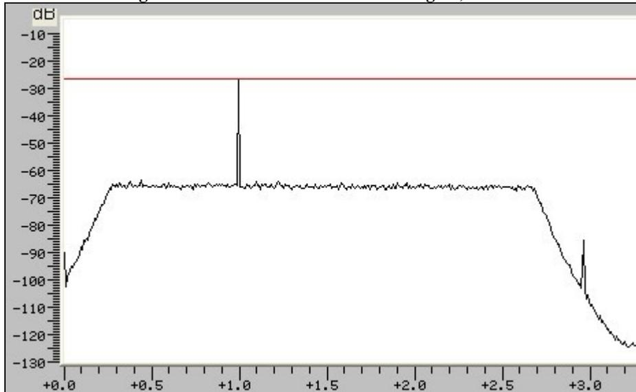
Figure 8: SSB 2.4 kHz. -120 dBm RF signal, max. NR (55%).
