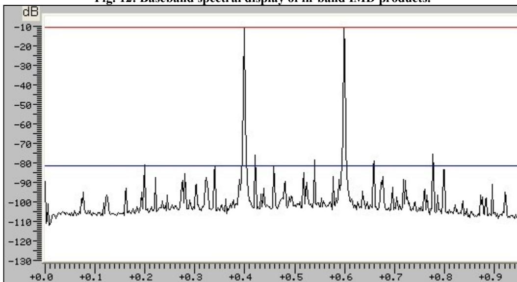
On the X-axis, +0.0 kHz  $\hat{=}$  9999.6 kHz (virtual carrier).  $f_1$  is at +0.4 kHz,  $f_2$  at +0.6 kHz. The 3<sup>rd</sup>-order IMD products are at +0.2 and +0.8 kHz respectively.
