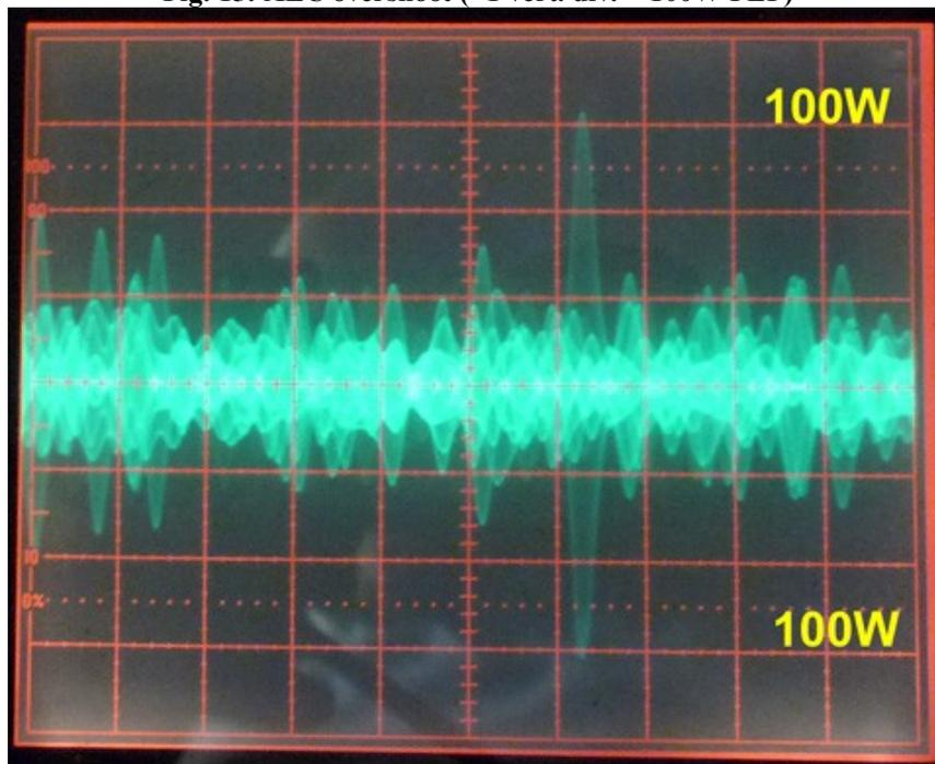
**18: Transmitter 2-tone IMD test.** In this test, a 2-tone test signal is applied to the USB port from a tone-generator program running on a laptop computer. A spectrum analyzer is connected to the IC-7410 RF output via a 60 dB high-power attenuator. The -10 dBm reference level equates to 100W.
