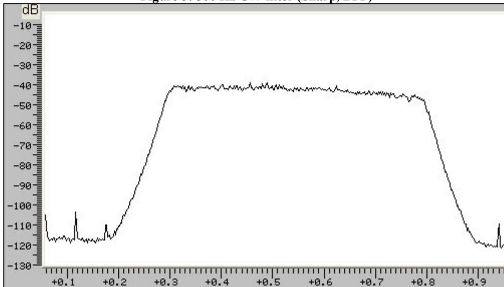
**Fig. 4: 500 Hz CW filter (Sharp, non-BPF)**
