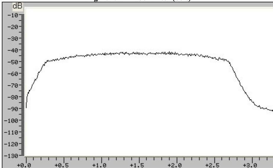
**Figure 3: 500 Hz CW filter (Sharp, BPF)**
