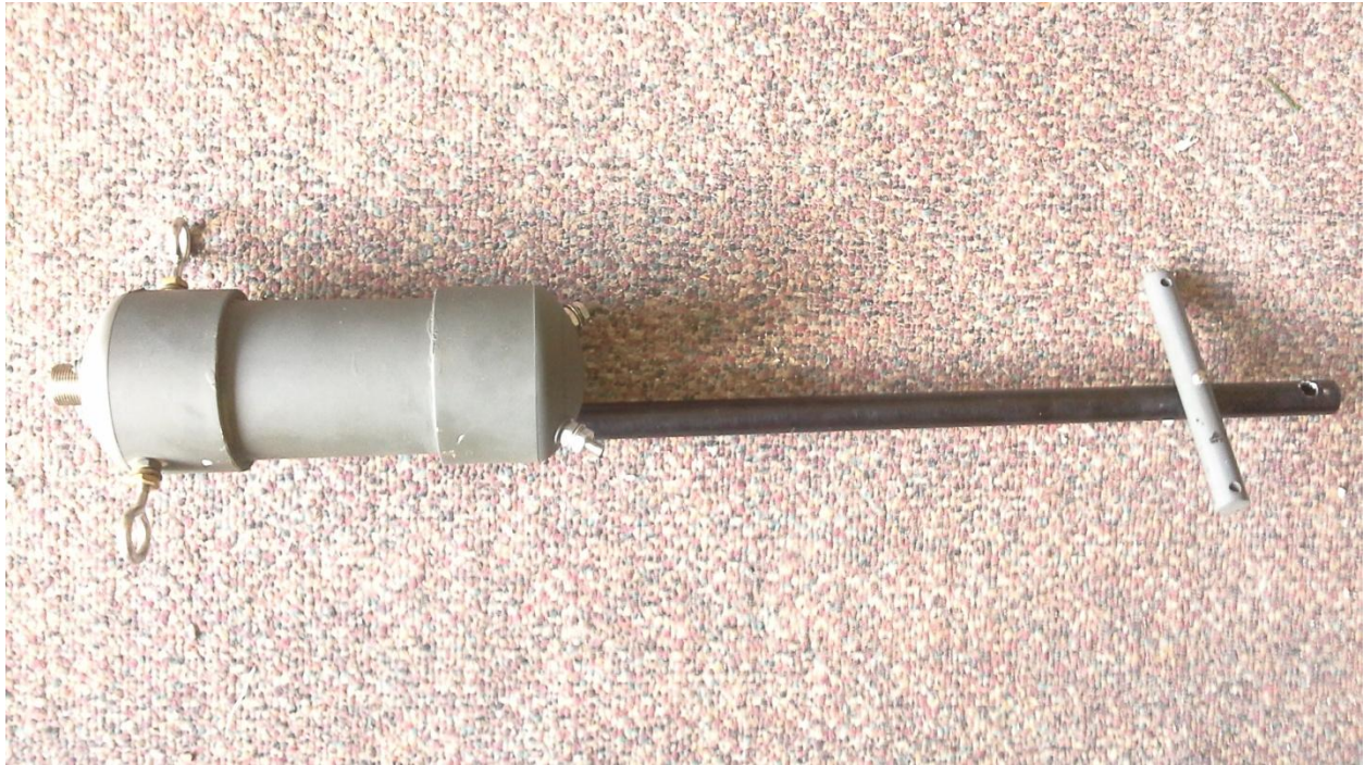
Attached spreader and insulator to the Balun termination assembly
