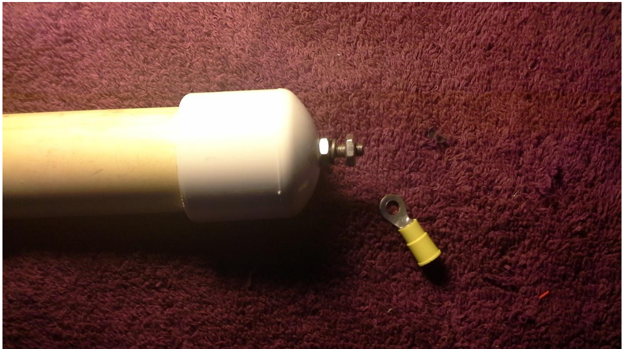
This is one end of the Termination Resistor pipe and Ring Lug. Hold the cap in place with a stainless screw and seal the cap with tape or coax seal. Also use coax seal on the bolt and ring lug and drill drain holes.
