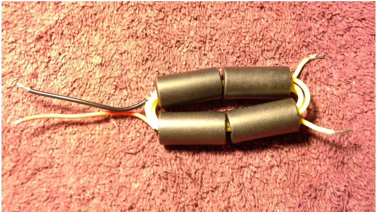
The original KISS Balun with 4 turns through the cores for 16:1 ratio.
