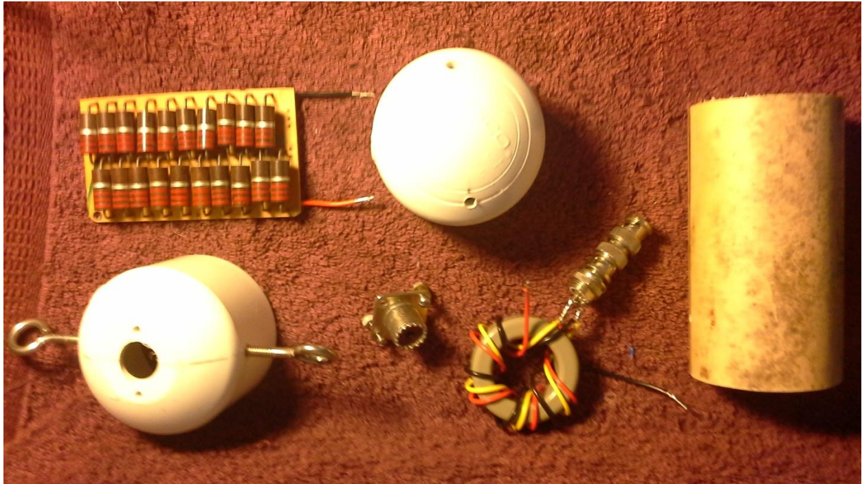
Beginnings of a 9:1 Balun and 450 Ohm Termination center assembly for 2 leg T2FD
