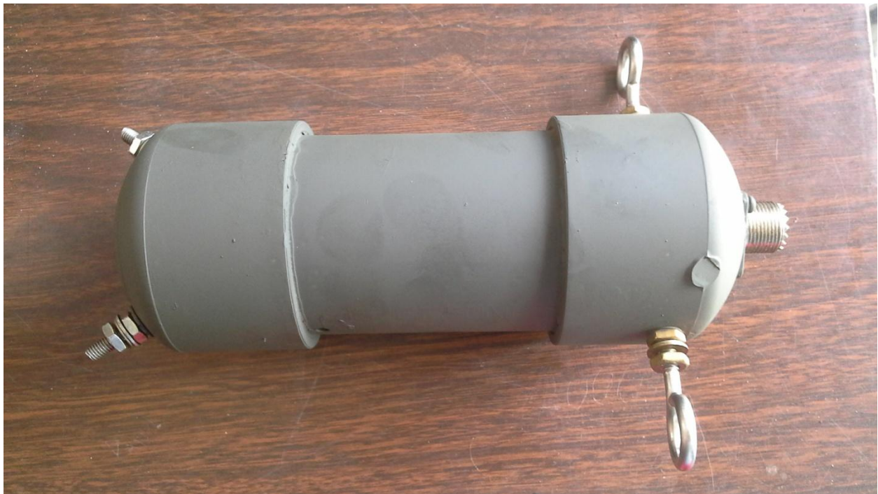
Finished Balun Termination assembly. I learned not to glue things together!
