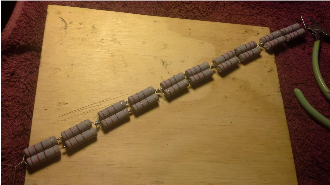
Termination Resistor Array (Note: This has 5 banks of 4, we want 4 banks of 4 resistors)
