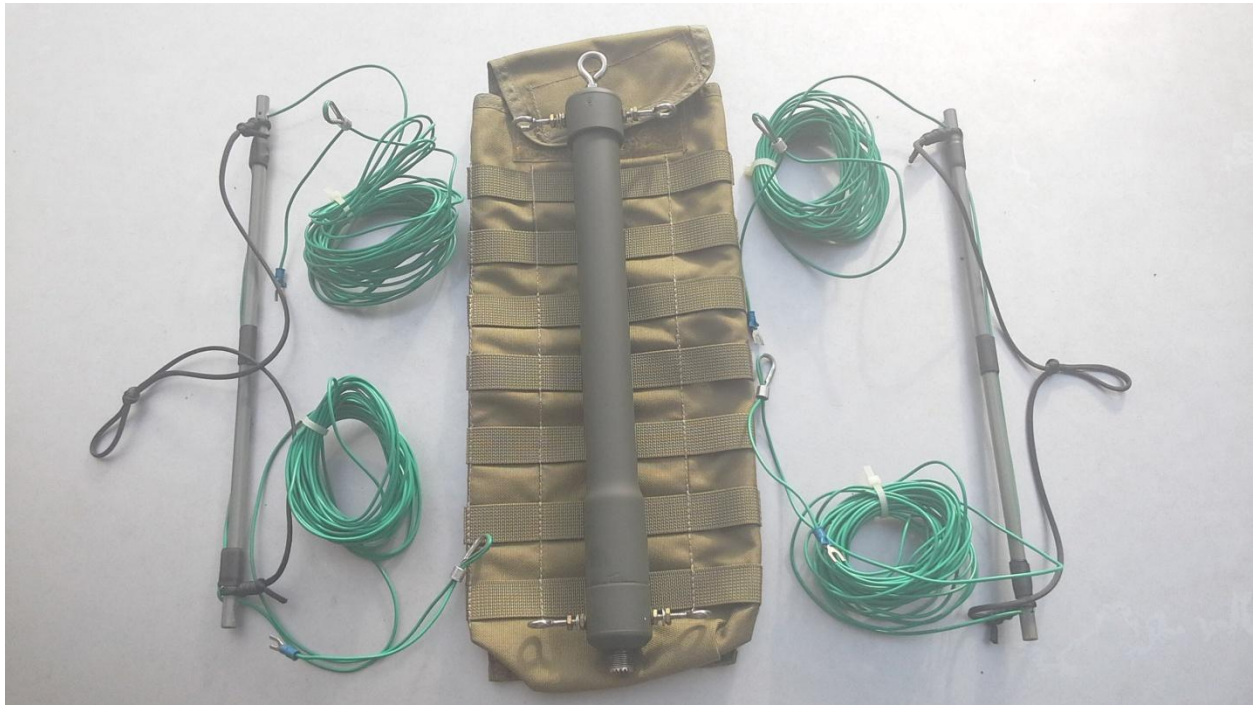
Portable T2FD Antenna fits in Hydration Bag. Spreaders are made from fiberglass tent poles.
