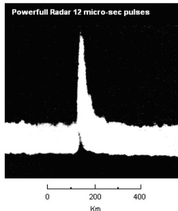
Fig.2 reflections observed from the moon employing a powerfull radar using 12 micro sec. pulses. The short range extent of the signal spectrum confirms that the reflections are largely from the center of the visible disk. The Graph is taken from this document: "Radio communication via the Moon" by J.V Evans (COMSAT Laboratories-United States)
