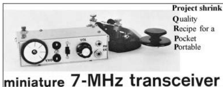
achieved by switching in a 7uh coil in series with the VXO crystal. VXO range was about 4KHz, depending upon the activity level of the crystal.
