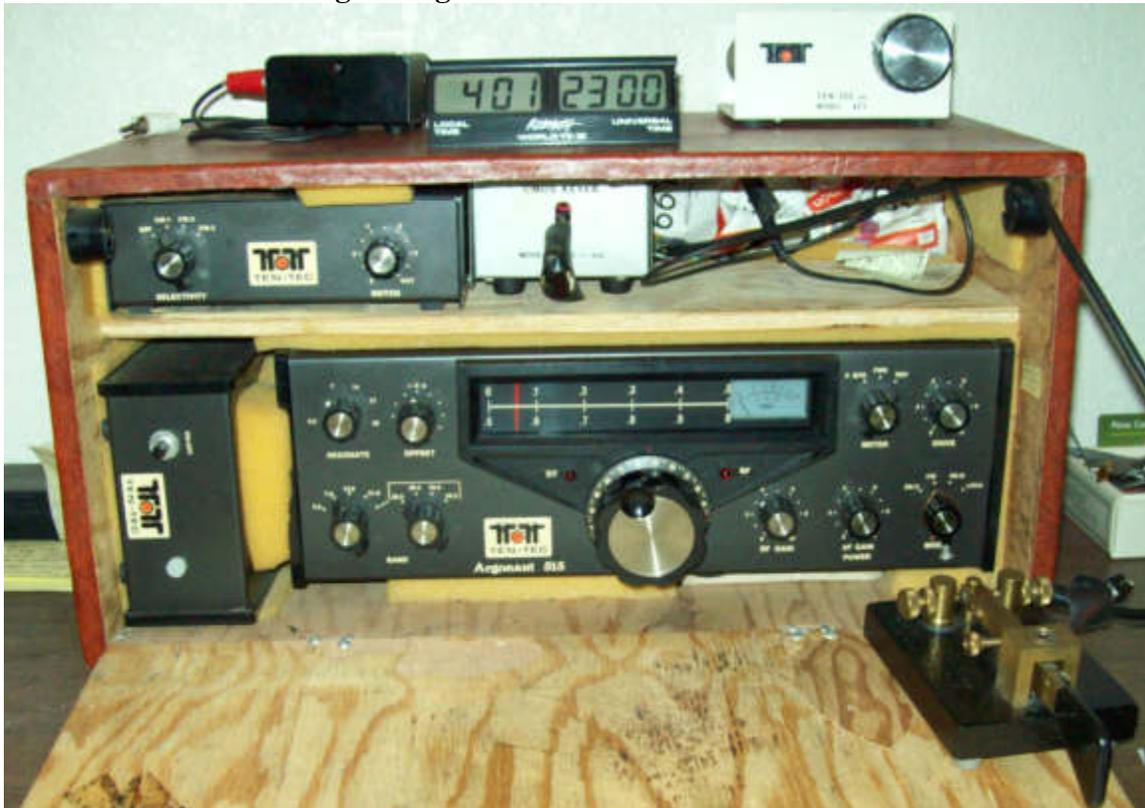
The “mobile travel box” was built specifically to fit the 515 station into the space between the front seat and dashboard on the transmission hump of my 1966 Pontiac
