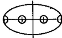
Divide the outer edge of the 4-1/2" circle into six parts (use the compass to scribe the 2-1/4" radius on the circumference of the circle to roughly divide it into six parts) and lightly connect the marks on the opposite edges through the center of the circle.
