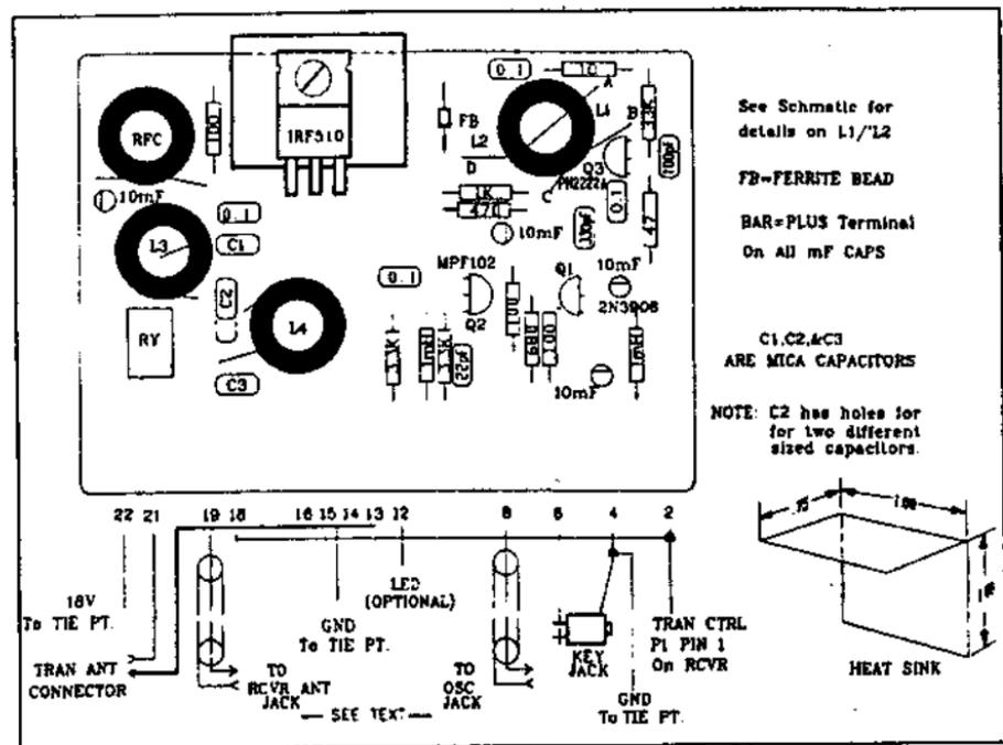
Fig. 15 Transmitter Board Component Side
