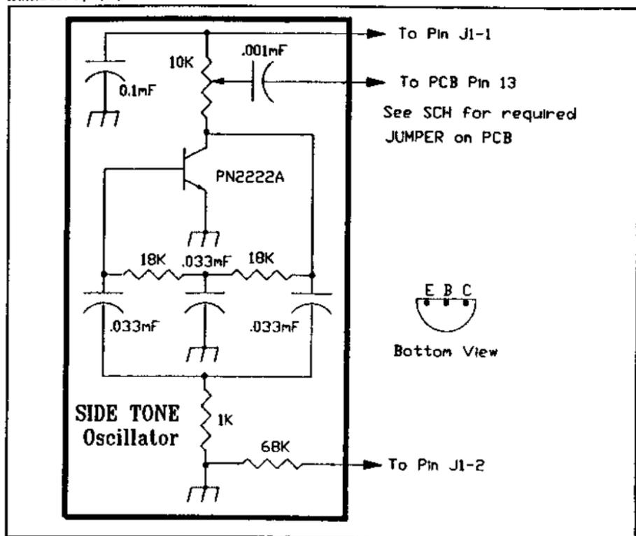
Fig. 16 Side Tone Oscillator Circuit
