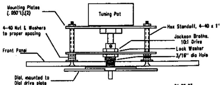
Note: 1) The most important part of this installation is to have the mounting plates parallel to the front panel to prevent binding of the tuning device. Thus, insure the spacer lengths are equal and that they are perpendicular to the panel.
