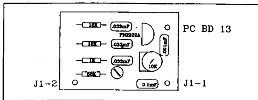
Fig. 17 Side Tone Oscillator Board, Component Side
