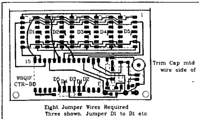
Fig. 13 Location of eight jumper wires that must be installed on the back of the frequency counter board.
