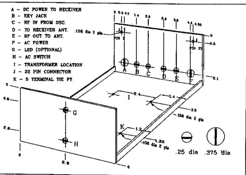
Fig. 8 Power Supply Chassis
