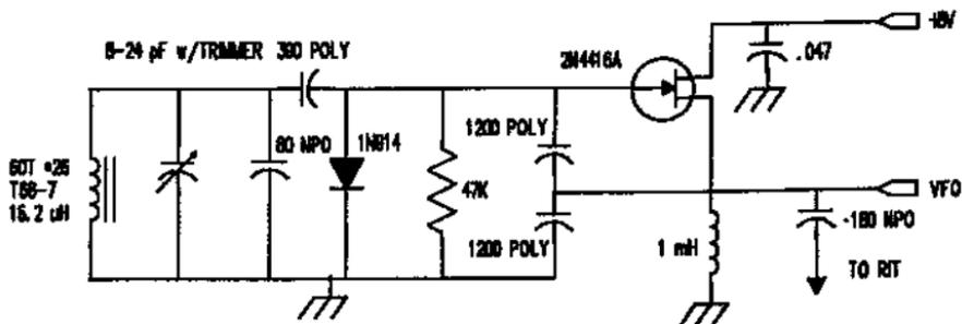
Schematic of Capacitor Tuned NC40 VFO
