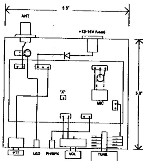
"X" - connector for external VFO and/or digital display
