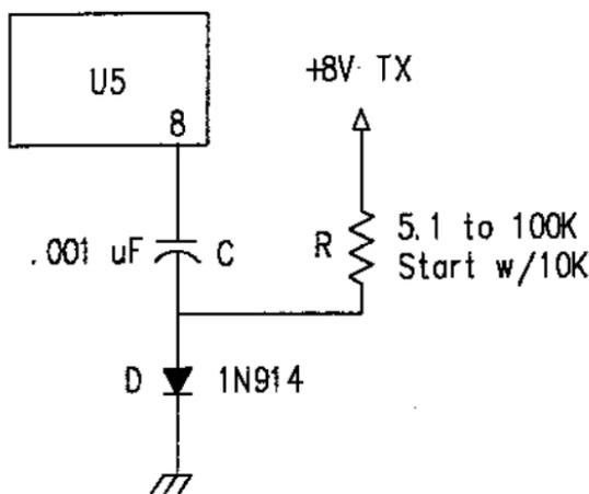
Don't cut any traces or remove existing parts: just add these three (R,C,D) to the existing circuit.
