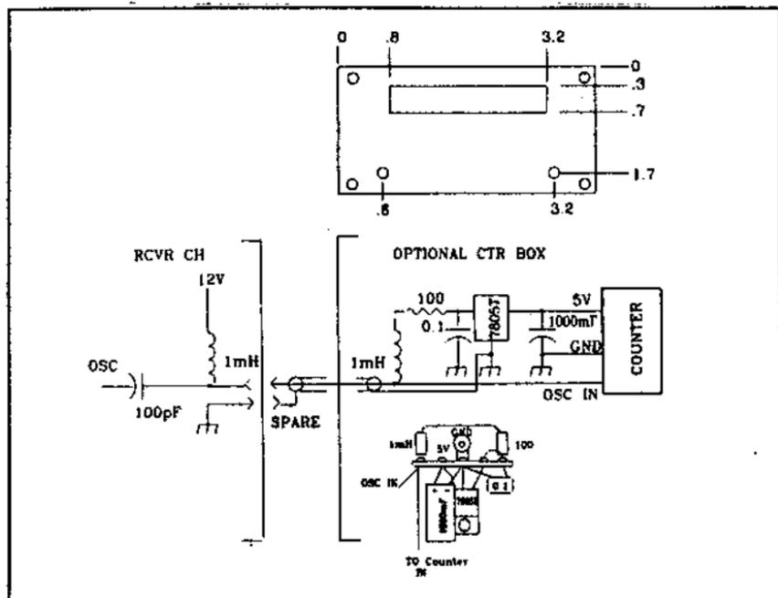
Fig. 3 Connecting Optional Frequency Counter
