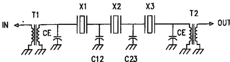
CE is the end capacitor (Cend from the program run above), C12 is the cap between crystal 1 and 2, C23 is the cap between crystal 2 and 3 and so forth. The values given for these caps are in picoFarads. The xformers are to bring the source and load impedances to 450 ohms (this \*IS\* important - if it's not at 450 ohms the filter won't behave well at all, with lots of ripple and poor rejection).
