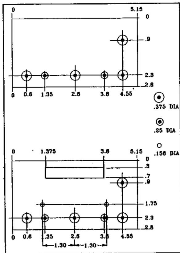
Fig. 10A Hole Template, Receiver Chassis
