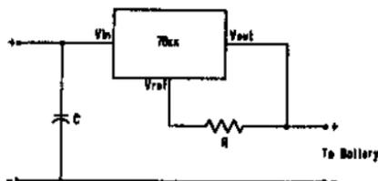
In this configuration, the 78XX regulator is a constant current source. The current to charge a NiCd is typically 10% per hour of its full amp-hour capacity. It will take 12 hours to charge a NiCd on this basis due battery losses.
