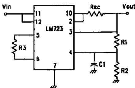
$$V_{out} = (V_{ref}) \times \frac{(R1 + R2)}{R2}$$
