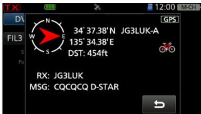
When you receive the signal, the RX position data is displayed in the RX position window.
