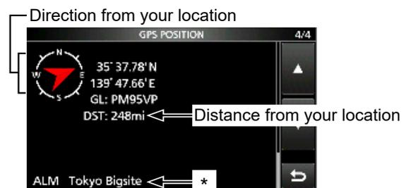
\* When a name is not entered in the GPS Memory channel, date and time are displayed instead of the name. In the QUICK MENU screen, you can change the GPS Memory or GPS Alarm in the GPS POSITION screen. (p. 12-6)
