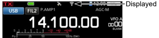
① The transceiver automatically connects to the last connected AP when the transceiver is turned ON.
