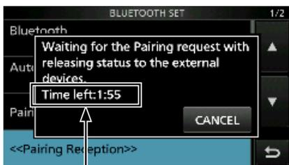
Turn ON Bluetooth with your Android device within the displayed period of time. When the time runs out, the transceiver exits the Pairing Reception mode.
