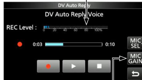
Touch to open the MIC GAIN adjustment window.
