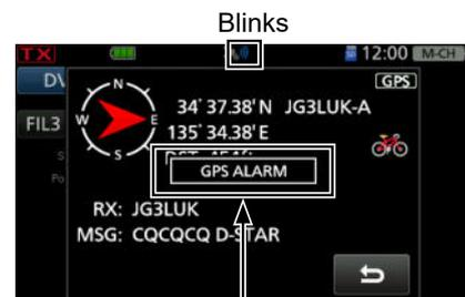
“GPS ALARM” pops up on the screen and the alarm sounds 3 times.
