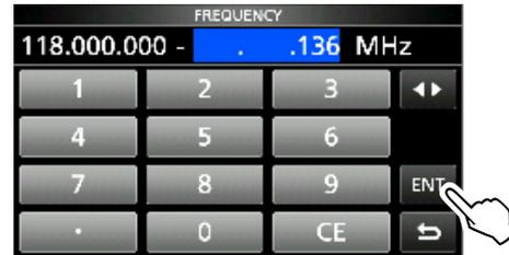
① Touch **◀▶** to select the upper and lower edge frequency, and then rotate **⊕MULTI** or touch the keypad to edit the frequency.
