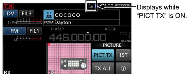
2. Push **(TRANSMIT)**, or hold down the microphone's [PTT] to transmit.
