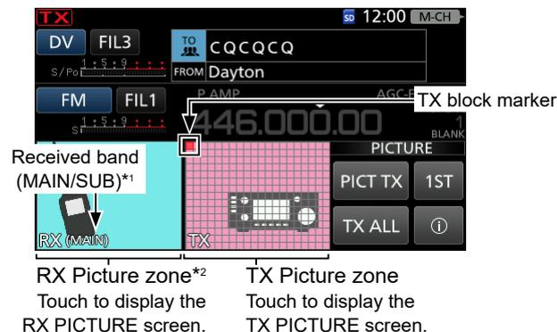
\*1 Displayed when using the transceiver with Dualwatch function.
